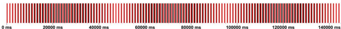
Figure 5: Bar chart of the last example with a least common multiple (lcm) of 142.780 ms (2,4 min) and a release level of 38%. The red and black bars represent two different transceivers. The period length and pulse lengths are shown downscaled.
