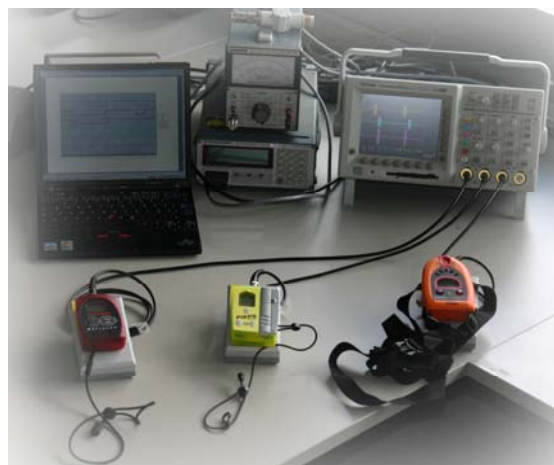
Figure4: test arrangement with three receiver modules, a storage oscilloscope (Tektronix TDS3014B)
