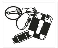
In order to use the Barryvox for searching, open the red buckle on the front. The beacon remains firmly attached to the harness system/body by the snap hook or to the wrist/body by means of the wrist strap. Adjusting the length of the wrist strap (quick catch) facilitates comfortable use. If you carry the Barryvox in your trouser pocket, make sure the pocket's zipper is closed throughout the tour. Sewn-on pockets are not suitable.
