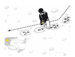
Do an accurate direction adjustment before the direction arrow disappears! You are then moving to the transmitting beacon in best coupling position and save time during the cross-like movements.
