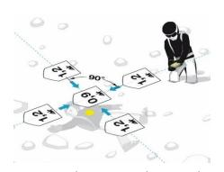
Move your beacon at a slow, steady speed of about 10 cm/s, keep it leveled close to the surface and do not rotate your device. Search along the Y axis, determine the lowest distance value, then follow along the X axis. Always move past the point of the lowest distance to verify the distance tendency. Mark the point of the lowest distance reading and start pinpointing.
